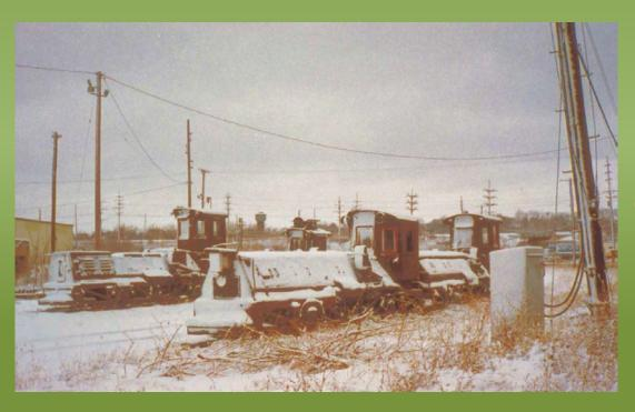
Shunt engines were used to move the rail cars under the Hulett Ore Unloaders for filling with iron ore
