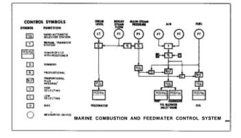
The automated wide-range combustion and feedwater control system installed in the *Mather* separated the fuel-air ratio into two subloops; (1) oil flow controlling, and (2) air flow controlling.
